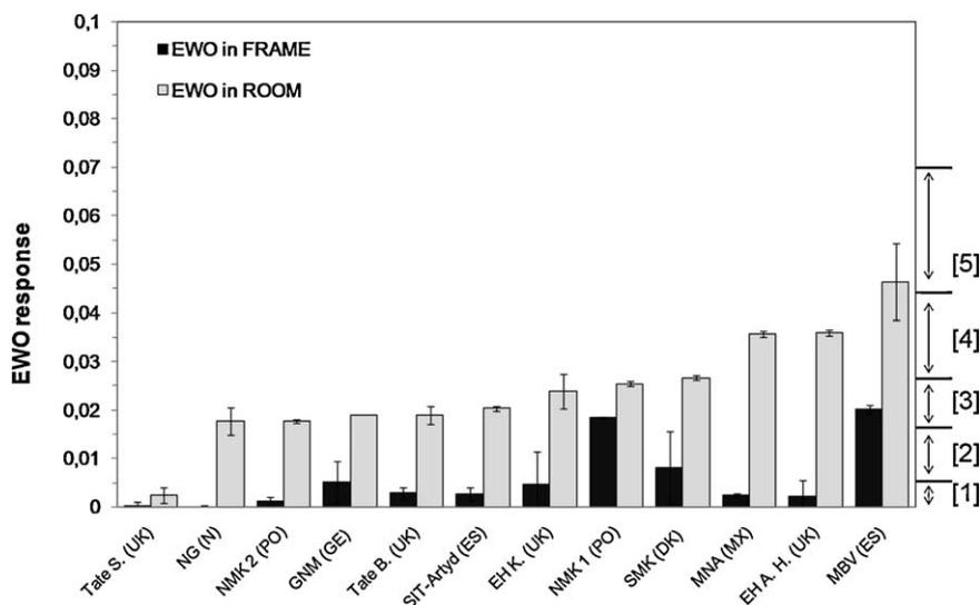
**Fig. 2.** Results from Early Warning Organic (EWO) (average of two parallel exposures, except in GNM room, absorption units at 340 nm). SMK = SMK1. Number in brackets are tolerability location levels [11] (at relative humidity  $H = 55\%$ ): [1]: Archive store, [2]: purpose built Museum Gallery, [3]: Historic House Museum, [4]: Open display in open museum, [5]: Outside store with no control.
