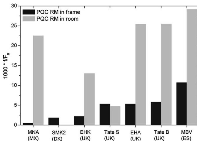
**Fig. 3.** Results from Resin Mastic Piezoelectric Quartz Crystal (RM-PQC).  $f / F_0$  = relation between the frequency shift and the original coated crystal frequency (KHz). For SMK2 measurement was not performed outside the mc-frame. The standard deviation for the measurements ranged from 0.66 to 1.0 with unit  $1000 \times f / F_0$ .
