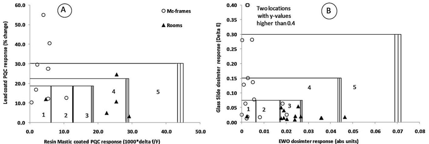
**Fig. 8.** Location-tolerability diagrams with threshold values (Fig. 2) for cultural heritage objects in indoors locations. A. Results from Resin Mastic Piezoelectric Quartz Crystal (RM-PQC) (x-axis) and Lead Piezoelectric Quartz Crystal (L-PQC) (y-axis) (Figs. 3 and 4) and B. from Early Warning Organic (EWO) (x-axis) and Glass Slide Dosimeter (GSD) (y-axis) (Figs. 2 and 5). The close vertical lines are the relative humidity dependence for each level.
