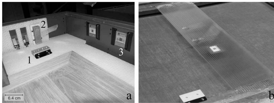
**Fig. 1.** Three dosimeters: 1. Early Warning Organic (EWO) dosimeter. 2. Resin Mastic (RM-PQC) and Lead Piezoelectric Quartz Crystal (L-PQC) and 3. The Glass Slide Dosimeter (GSD), mounted inside the “modern” SIT-Artyd mc-frame (a) and a “historic” frame adapted to mc-frame at The National Gallery, Oslo (b).
