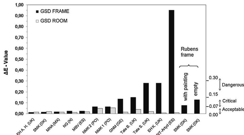
**Fig. 5.** Results from Glass Slide Dosimeter (GSD) ( $\Delta E$  - Extinction values measured as IR absorption at  $3300\text{ cm}^{-1}$ ). (SMK = SMK1). Numbers in brackets are GSD impact levels: (1'): acceptable, (2'): critical, (3'): dangerous.
