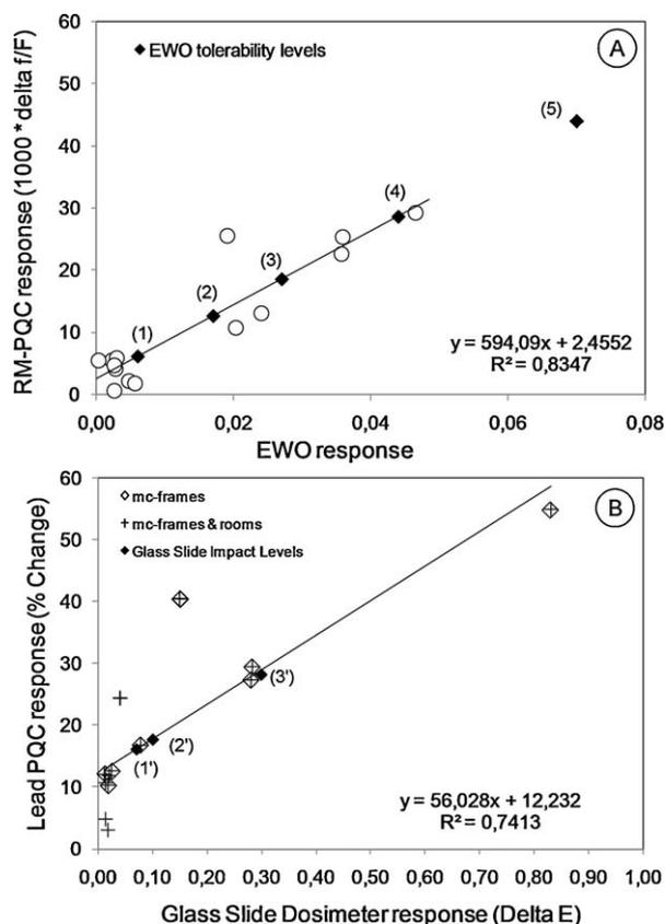
**Fig. 6.** Correlation between dosimeter responses in mc-frames and rooms. A. Early Warning Organic (EWO) and Resin Mastic Piezoelectric Quartz Crystal (RM-PQC) with locations tolerability levels (Fig. 2). B. Glass Slide Dosimeter (GSD) and Lead Piezoelectric Quartz Crystal (L-PQC) with impact levels (Fig. 5).
