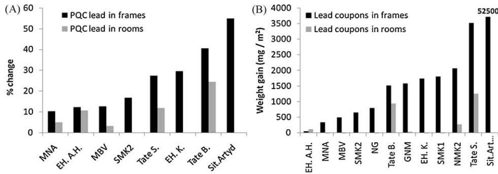
**Fig. 4.** A. Lead Piezoelectric Quartz Crystal (L-PQC) (Change (%) in frequency or mass) for selected site exposures: B.L lead coupons (weight gain / unit area) for site exposures. In the case of SMK2, EH.K and SIT-Artyd, measurements with L-PQCs were not performed in the rooms. For the other rooms no response was detected. The standard deviation for the measurements of the L-PQCs ranged from 0.12 to 0.22%.
