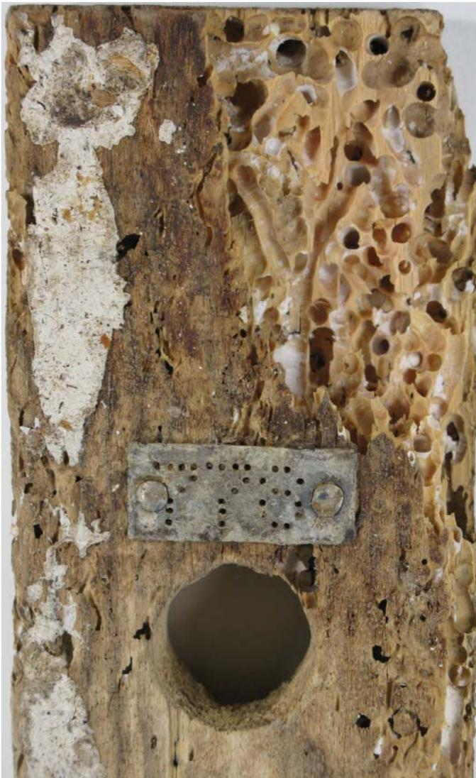
FIGURE 2 Heavy attack by *Teredo navalis*. The mollusc penetrates and digests the wood material forming up to 1 cm wide tunnels.
