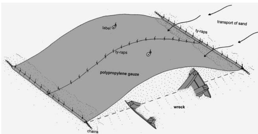
FIGURE 6 A method using sediment transport and a porous net to cover a wreck with sediment and preventing attack by shipworm.
