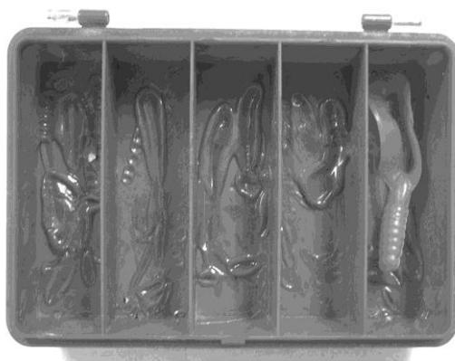
Figure 5. A polyethylene fishing box has absorbed plasticizer from plasticized PVC lures and formed polyethylene 'fossils' over 20 years
