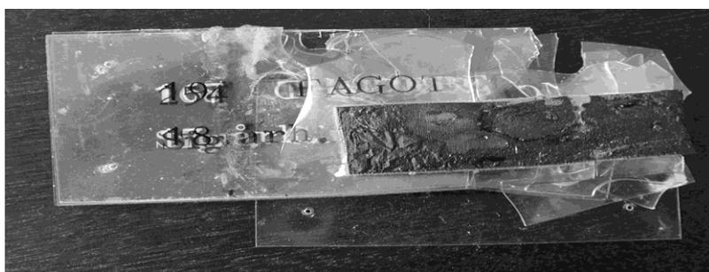
Figure 1. Poster from Museum of Historical Music in Copenhagen, Denmark made from cellulose nitrate in the 1960s shows shrinkage and tackiness due to loss of plasticizer and crizzling of the polymer.
