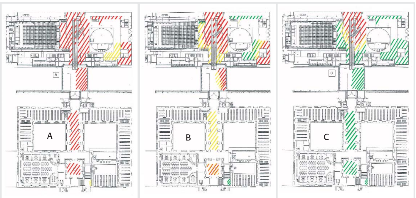
10 Ground map with colour marking for the three different light sensitivity categories: extremely light sensitive objects (A); highly light sensitive objects (B); medium light sensitive objects (C). The red marking indicates exhibition is recommend for less than 3 weeks. The yellow markings show areas for exhibitions less than 3 months. The green markings from 3 months and upwards.
