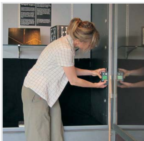
4 Photometric measurement at the Bigger Queen exhibition case. Measurement taken without glass to be compared with measurement when the glass front is closed.
